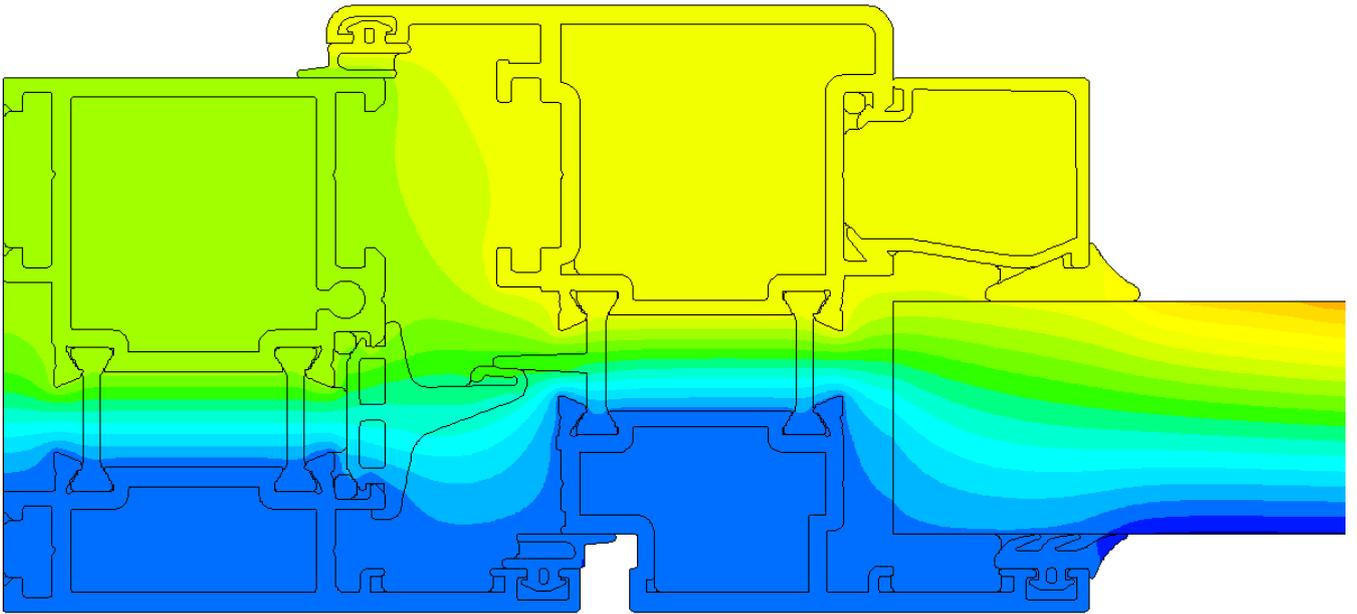
Figure 2. Isotherms (colour increment of 1°C, line increments of 1°C and 5°C)
