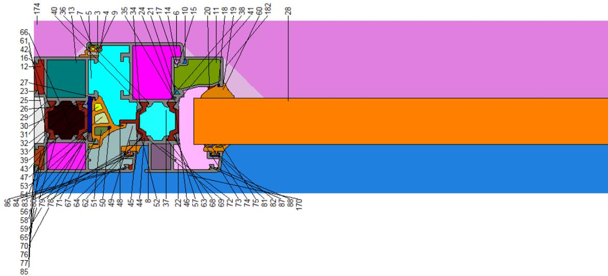
Figure 1. Frame section (with colour numbers)
