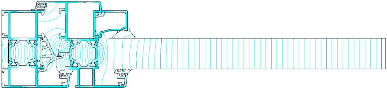
Figure 3. Heat flow lines (increment 0.1 W/m).
